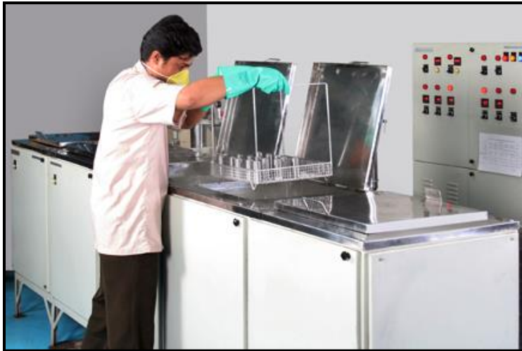
5-Tank Ultrasonic cleaning system for part cleaning
