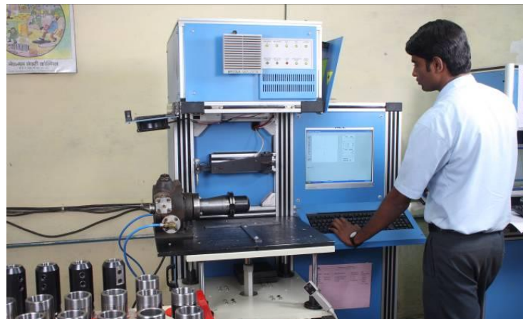
Laser Marking of Batch Number on Each Holder for Traceability
